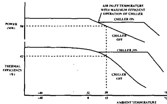
FIGURE 11: Typical Uninstalled Industrial Trent Performance Data
